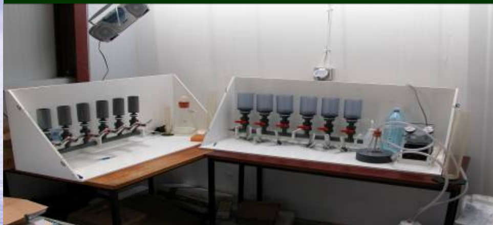
Custom built filtration systems
